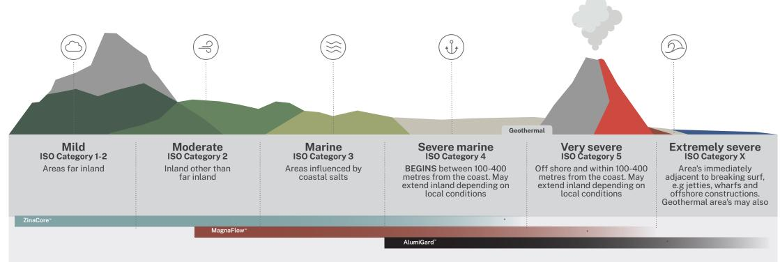
Buildings with exposure to corrosive chemicals such as airports, gas stations, fertiliser or dairy factories may require the ColorCote® 'Plus' paint system to ensure roof or cladding is better protected from chemicals in the environment. Please contact ColorCote® for a recommendation if you are unsure which paint system is required.
