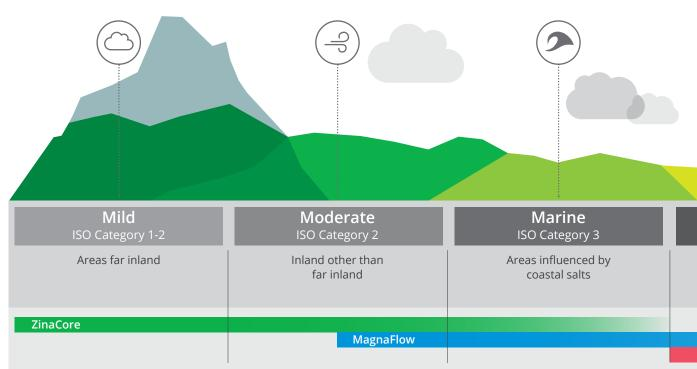
Buildings with exposure to corrosive chemicals such as airports, gas stations, fertiliser or dairy factories may require the ColorCote 'Plus' paint system to ensure roof or cladding is better protected from chemicals in the environment. Please contact ColorCote for a recommendation if you are unsure which paint system is required.
