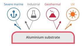
The outer layer is an acrylic or polyester top coat baked on a polyester primer, resisting UV damage for outstanding colour and gloss retention. While the purchase and installation costs of AlumiGard are higher, it has considerably greater durability than steel, giving you decades of worry-free protection in the harshest environments.
