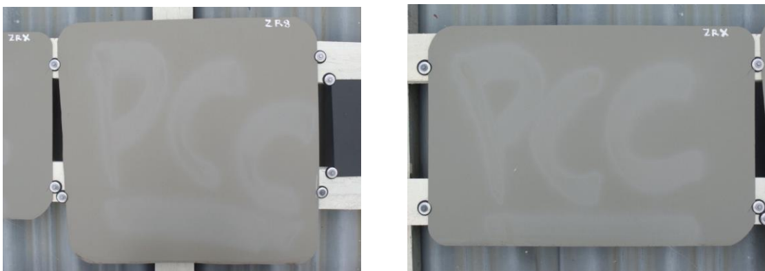
Fading effects of spray paint on ColorCote Zinacore & ZinacoreX™ – just 18 months after installation
